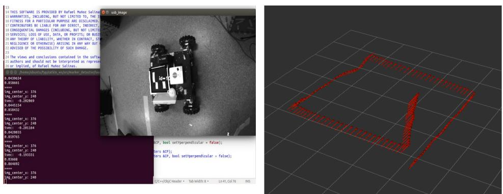
In joint testing, missions can be executed in order defined in flight logic. After taking-off, UAV was firstly sent out for target searching, and then UGV moves to the target automatically with UAV following it. Meanwhile, PID controller and EKF are running in the background. The EKF is able to propagate and update robot positions in relatively high accuracy (0.3m).
