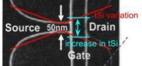
Measured as the percentage of variation with respect to gate length, the significance of both structural deviations on finFET performance are compared. The underlying effects in the subthreshold region is analysed based on the potential profile. Statistical study is also conducted to assess the performance variation in response to different degrees of gate misalignment.
