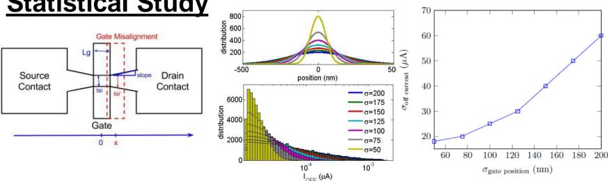
Based on a Gaussian distributed gate position and a pre-determined mapping of gate position to a modified fin-width and its tapering slope as shown in the figure above, it is shown that the distribution of off-current responds similarly to the underlying gate misalignment-distribution. This can also be seen from the positive relationship between the two standard deviations.
